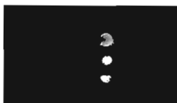
Figure 1. The O 2 concentration distribution images of the three-tube phantom containing LiPc radicals.
